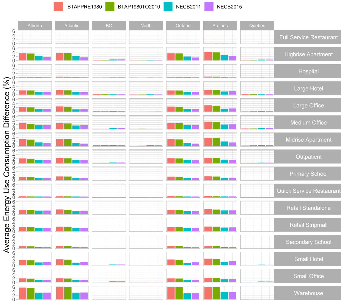
Figure 2. Marginal percentage energy use intensity increment for various building archetypes and vintages in regions across Canada
