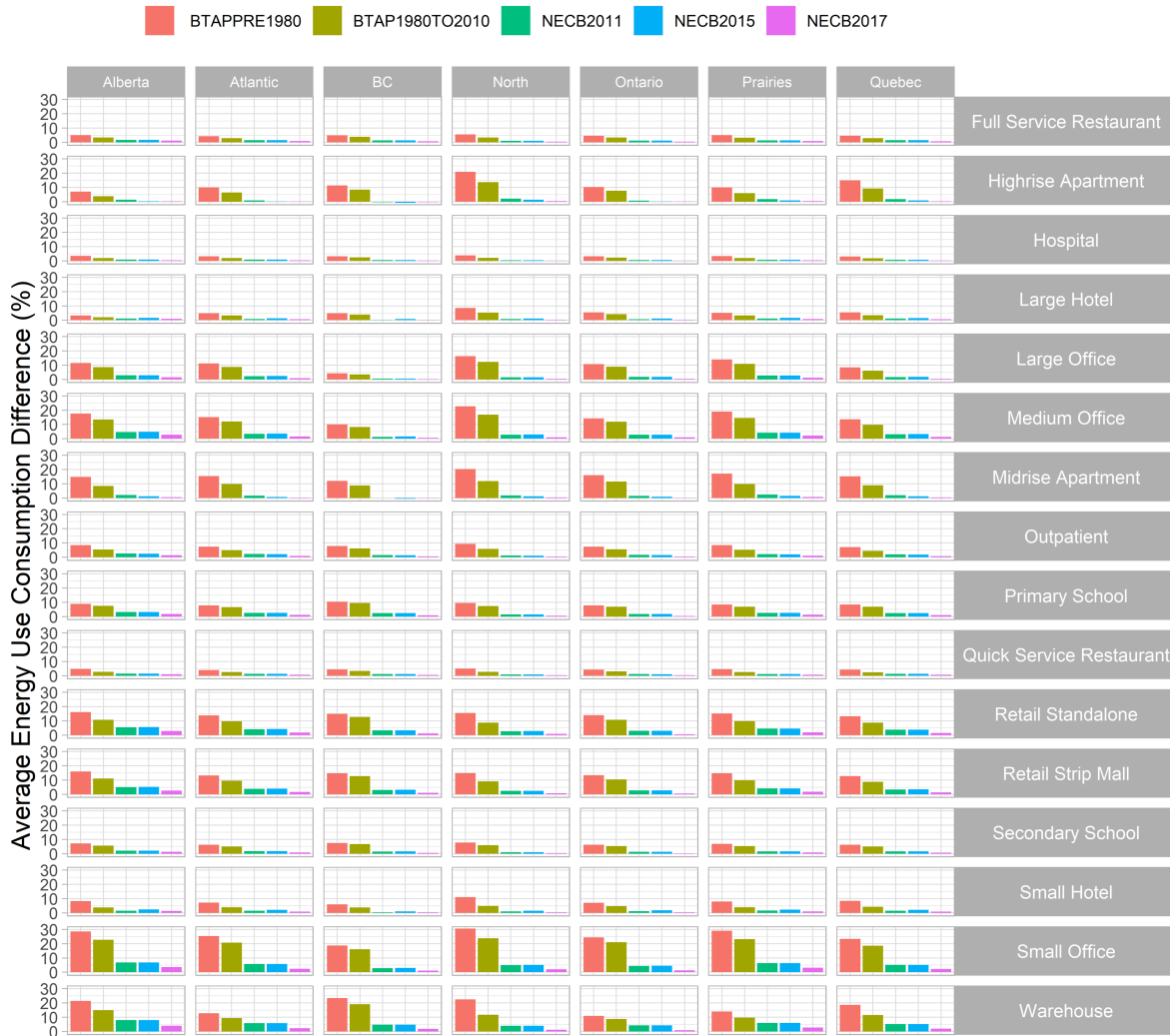
Figure 2. Marginal percentage energy use intensity increment for various building archetypes and vintages in regions across Canada
