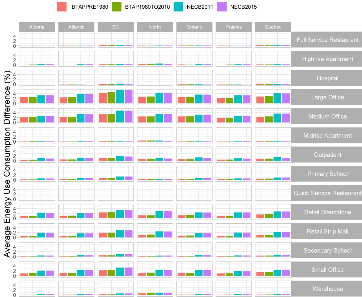
Figure 3. Marginal percentage energy use intensity increment for various building archetypes and vintages in regions across Canada
